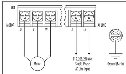
**5.2 Ground Connection** – Connect the Ground Wire (Earth) to the Green Ground Screw. The Ground Screw is located next to Terminal Block TB1. See Figure 6 on page 13.
