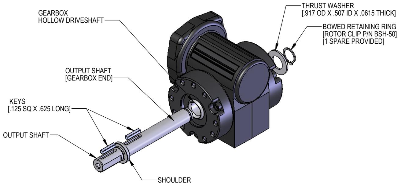
1. Insert key into keyway on gearbox end of output shaft.
