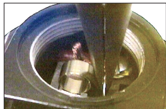
Figure 4 – Grasp spring with pliers.
