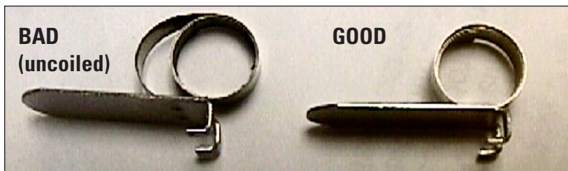
Figure 11 – Comparison of bad and good springs.
