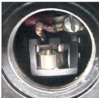
Figure 13 – Coil centered directly over brush.
