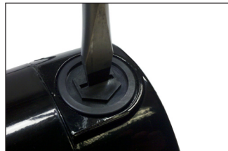
Alternate brush cap may be removed with a 3/4" hex wrench
