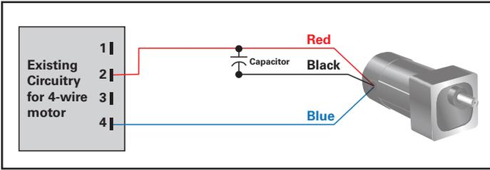
**Figure 3: Three-wire non-reversing connection (clockwise direction of rotation when viewing output shaft)**
