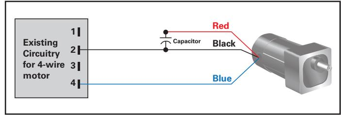
**Figure 4: Three-wire non-reversing connection (Counterclockwise direction of rotation when viewing output shaft)**
