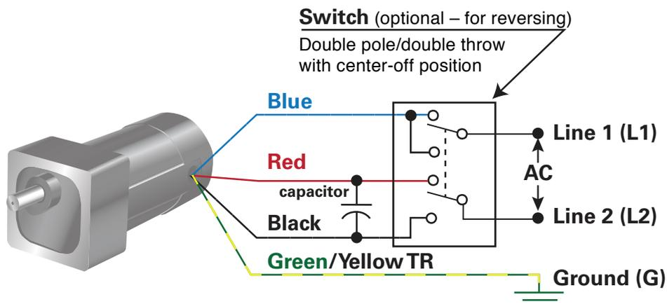
**4-Wire Bodine AC Motor or Gearmotor**
