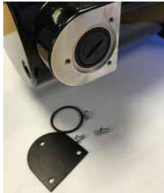
Remove the metal brush cap shield and the rubber O-ring beneath it.
