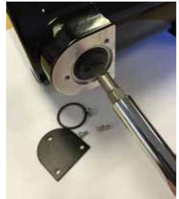
Remove the plastic brush cap with a large slotted screwdriver.
