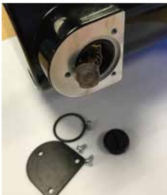
When the brush cap is removed, the brush spring will pop out.
