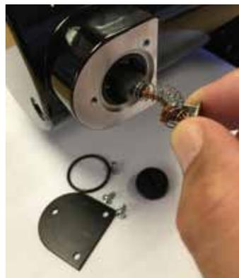
Grab the spring and remove the old brush assembly from the brush holder.
