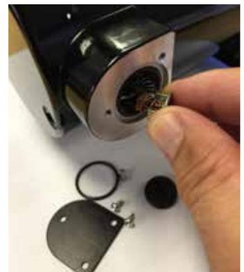
Reverse the order of these steps to install the new parts. Guide spring coils into holder and secure metal tab flush with brass insert before installing threaded brush cap. Install O-ring and brush cap cover plate.
