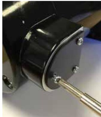
Remove the 3 screws with a small Phillips head screwdriver.
