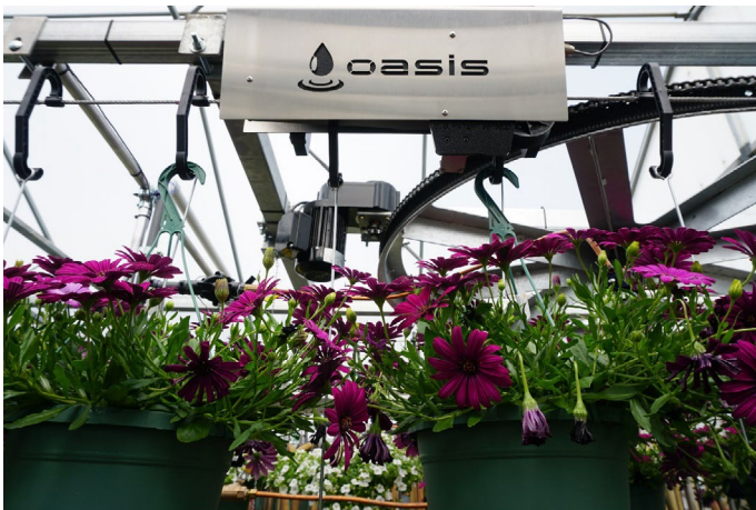
An inverter-duty gearmotor drives a conveyor that carries hanging flower baskets under a water sprinkler in a greenhouse. By adjusting the gearmotor speed slower or faster, the flowers receive more or less water. (Image: Control Dekk)
