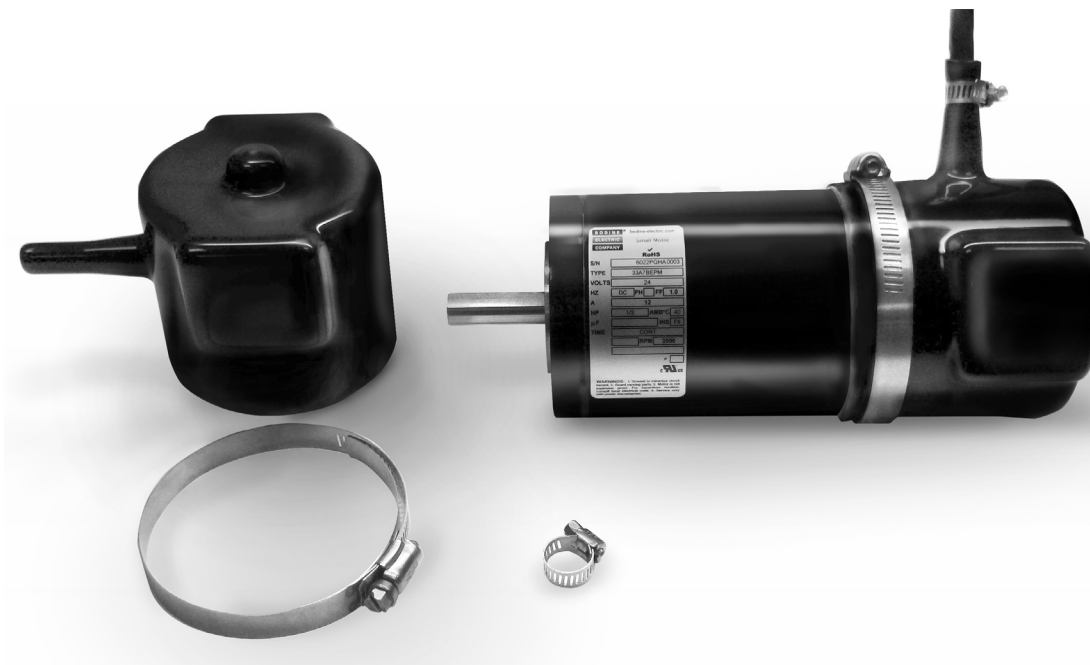
Figure 5: A Brush DC motor with a vinyl boot covering the end of the motor to protect the lead exit and cover the brush caps from water ingress.
