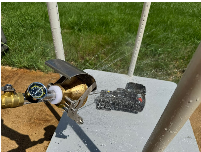
Figure 3: A gearmotor being tested for the IP44 standard.
