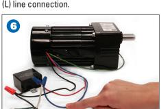
Connect the other side of the AC line. Connect the blue motor lead to the other lead of the AC line cord. Again, the connection may be made to either side (i.e. hot or neutral) (Figure 6).
