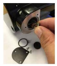
Reverse the order of these steps to install the new parts. Guide spring coils into holder and secure metal tab flush with brass insert before installing threaded brush cap. Install O-ring and brush cap cover plate.
