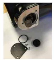
When the brush cap is removed, the brush spring will pop out.
