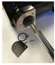
Remove the plastic brush cap with a large slotted screwdriver.
