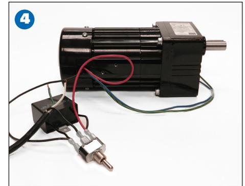
**Proceed to connect the blue motor lead to the other side of the AC line. To complete wiring, connect the motor's green-yellow ground lead to the ground on the AC line.**
