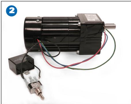
**Connect the black motor lead to one lead of the capacitor.** The capacitor is not labeled with polarities, so the connection may be made to either wire. **Next, connect to the "throw" end of the single pole, double throw switch.** The "throw ends" are normally the outer terminals of the switch (Figure 2).
