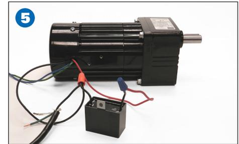
Since the wiring diagram does not specify AC line lead polarities, the connection may be made to either side of the AC line (i.e. hot or neutral) (**Figures 2 and 3**). However, when a switch is used it should interrupt the hot (L) line connection.
