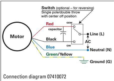
**PART 2: Wiring with a reversing switch (Wiring with a Single Pole, Double Throw Switch with Center-Off Position)**
