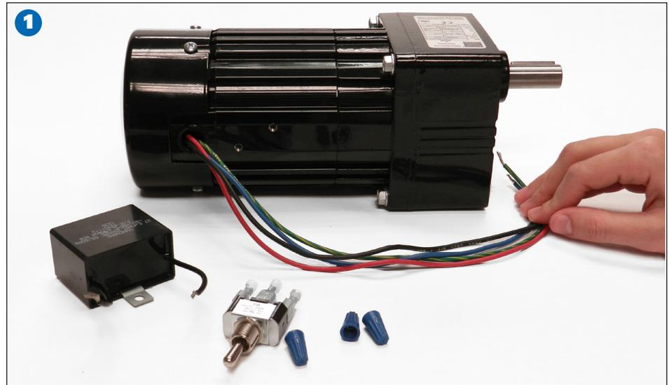
The purpose of the center-off position is to bring the motor to a complete stop before reversing its direction. Below are instructions on how to implement this diagram.
