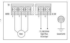
208/230 Volt AC line input with Jumper J1 set to the "230V" position (factory setting). Rated for 115 Volt AC line input with Jumper J1 set to the "115V" position. See Figure 6.
