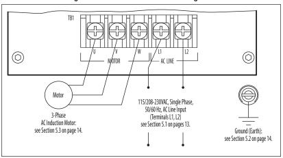
Figure 1 – Quick-Start Connection Diagram\*
