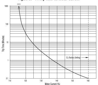
Figure 36 – I2t Trip Time vs. Motor Current
