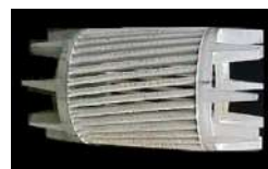
Fig. 2-8: Aluminum conductors in an AC induction rotor. The steel laminations have been removed to illustrate the "squirrel cage" form of the cast aluminum conductors
