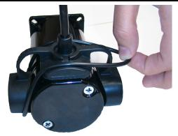
Slide O-ring over cord and position over brush ear and in topside channels. Stretch O-ring over opposite brush ear to secure assembly
