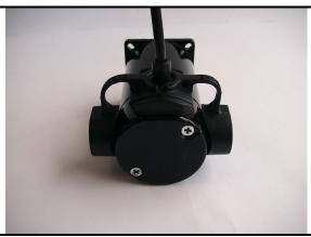
Press the rubber cover down tight against adhesive foam gasket. Push both brush ear covers over cast motor brush ears
