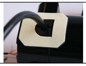
Peel off backing of either side of the foam gasket and attach to the motor over the strain relief
