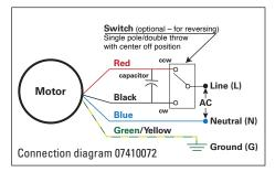
PART 1: Wiring without a direction switch Identify the wire colors and confirm that the gearmotor or motor is a 3-wire reversible PSC model. Bodine stock motors have red, black, and blue motor leads and a green-
