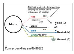
PART 2: Wiring with a reversing switch (Wiring with a Single Pole, Double Throw Switch with Center-Off Position)
