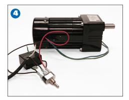
Proceed to connect the blue motor lead to the other side of the AC line. To complete wiring, connect the motor's green-yellow ground lead to the ground on the AC line.
