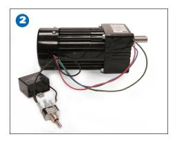
Connect the black motor lead to one lead of the capacitor. The capacitor is not labeled with polarities, so the connection may be made to either wire.
