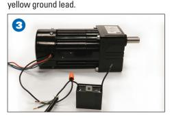
Since the wiring diagram does not specify AC line lead polarities, the connection may be made to either side of the AC line (i.e. hot or neutral) (Figures 2 and 3). However, when a switch is used it should interrupt the hot (L) line connection.
