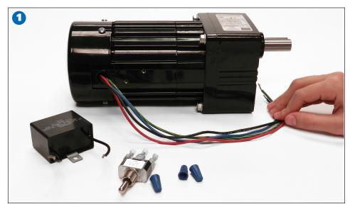
The purpose of the center-off position is to bring the motor to a complete stop before reversing its direction. Below are instructions on how to implement this diagram.
