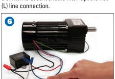
Connect the other side of the AC line. Connect the blue motor lead to the other lead of the AC line cord. Again, the connection may be made to either side (i.e. hot or neutral) (Figure 6).
